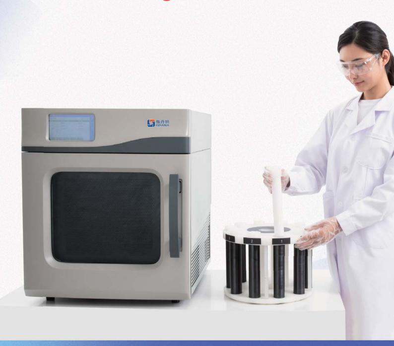
Microwave Digestion Instrument is an excellent assistant for elemental analysis techniques such as AAS,AFS,ICP,ICP-MS,as well as GC,HPLC,GC-MS,and other analytical methods. It offers highly efficient sample processing capabilities, capable of completing the digestion,extraction, protein hydrolysis, concentration, drying, and organic synthesis of the majority of organic/inorganic/liquid/solid samples within 20 minutes.
